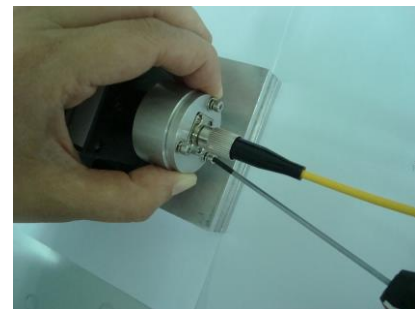
Figure 4-Checking laser output power
